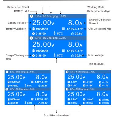
Rotating the roller wheel up or down during charging will switch the information displayed on the lower half of the LCD screen between cell voltage, cell IR and working parameters. Cell voltage and IR can only be displayed during the balance charging process.
